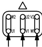
*Connection diagram for motors with one speed*
